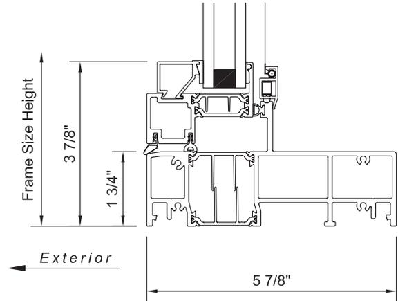
series 7660 awning and series 7670 casement window head - equal leg block frame
